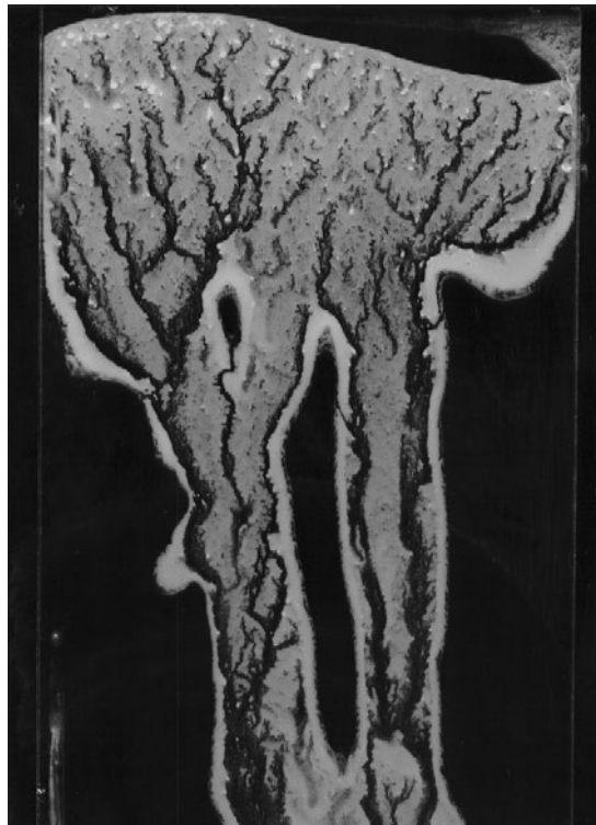
Figure 1. Digitized pattern of the flow of the yoghurt–water suspension over an inclined surface. The white areas are precipitated yoghurt, the black areas are washed by the flow of water. This is above the threshold angle in which we can see many global fractal trees.
